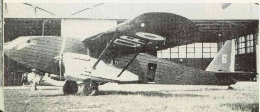
Developed from the Potez 540 'multiplace de combat', was the Potez 65 military transport, which employed the same wing, engine and tailplane design, but married to a new, capacious fuselage. Seen just before the war, this machine is serving with the 601e Groupe d'Infanterie de l'Air [paratroops].
