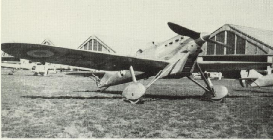
The excellent Dewoitine D.500, the first really modern French fighter, and a world trend setter, entered service in 1935. Distinguishable by its two-blade propeller, deep radiator and very wide undercarriage, this particular aircraft served with 2e Escadrille, GC I/1.
