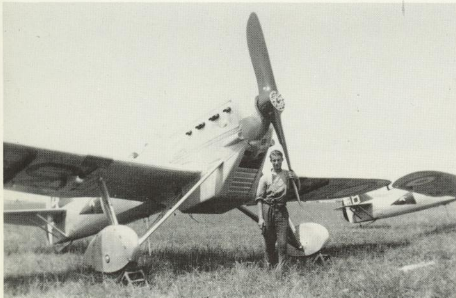
The D.501 differed from the D.500 only by virtue of the fact that a 20mm. Hispano 'moteur-cannon' was fitted between the cylinder banks of the engine, firing through the propeller boss. The muzzle can just be seen on this aircraft of 1e Escadrille, GC II/5. Photographed in 1937, it will be noted that these aircraft carry the famous 'Cigognes' [Stork] insignia of the 'crack' W.W.I Spad units.
