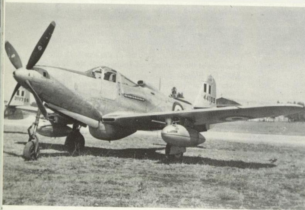
Late in the war a number of P-63 Kingcobras were received for ground strafing activities. This one served with GC II/9 'Auvergne'. Note the three long-range tanks, beneath wings and fuselage, and the underwing machine gun gondolas.
