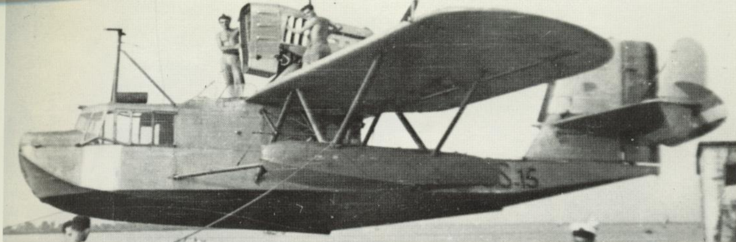
[Above] Widely used as a shipboard catapult aircraft, and for general coastal reconnaissance duties, the Loire 130 served with the Aéronavale in substantial numbers.
